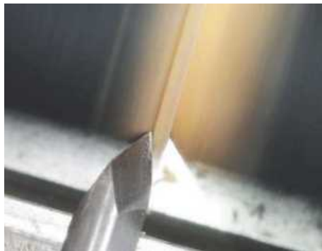
▲ Pic.11 If the tool is used correctly, you will only cut with the point of the chisel. If you start to see dust appear on the bevel of the tool, then you are very close to having a catch
